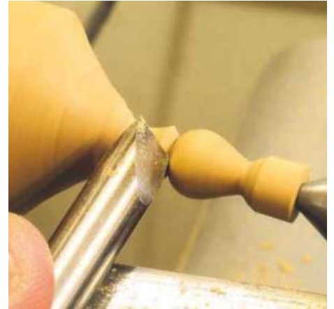
▲ Pic.21 The 10mm skew is being used to form the flame detail, which will be the top of the finial. Using the point of the skew will allow Les to get right into the tight detail
